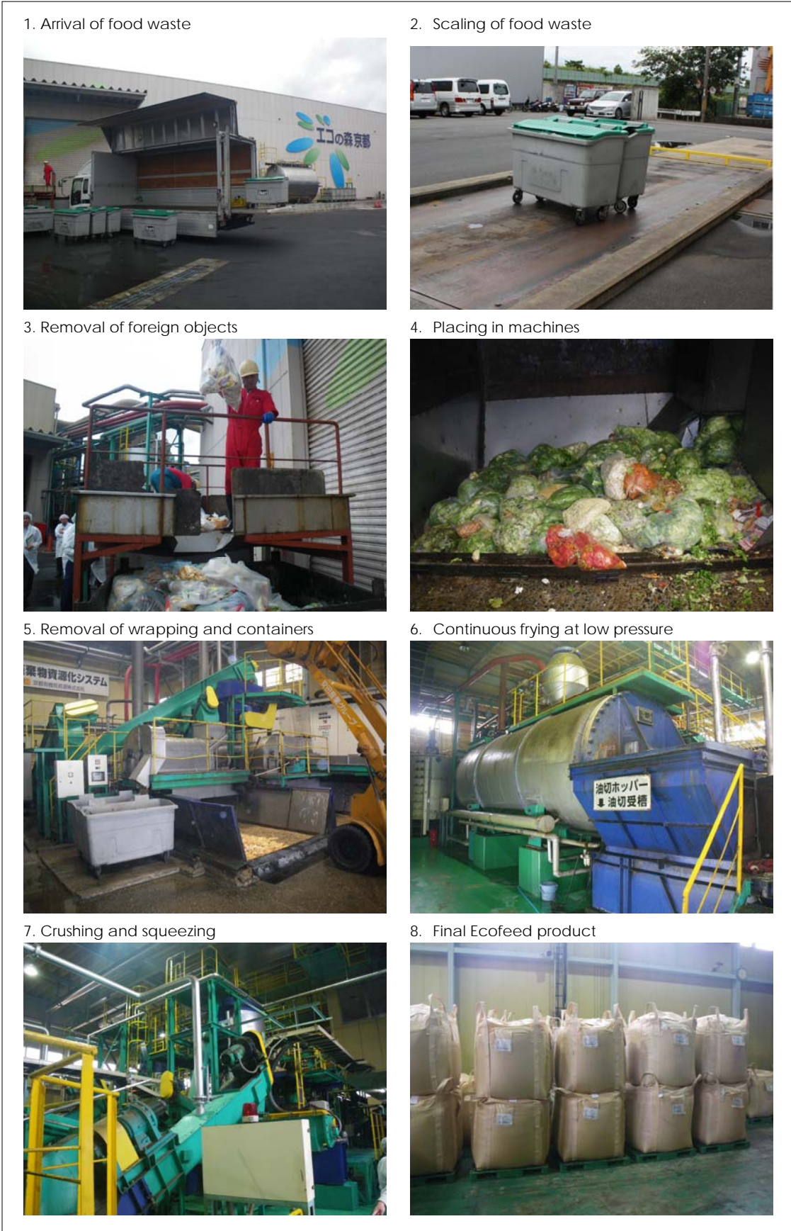
Figure 5 Examples of Ecofeed production procedures Photos: Courtesy of Kyoto Yukishitsushigen Co., Ltd
