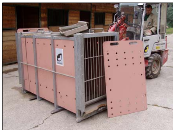
Figure 5 Crate for bears and big cats such as the cheetah that meets container requirement 73 of the International Air Transport Association Live Animal Regulations
