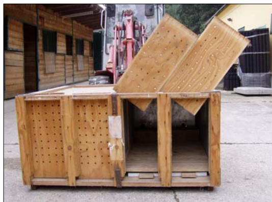
Figure 8 Crate suitable for canids such as the African wild dog ( Lycaon pictus ) according to requirement 82 of the International Air Transport Association Live Animal Regulations
