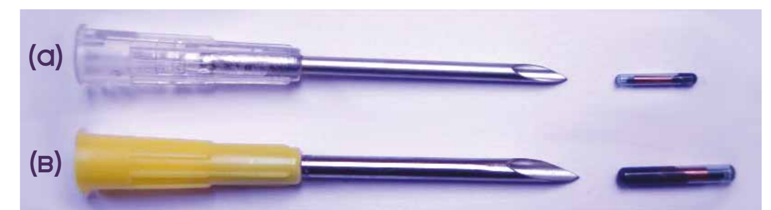
FIGURE 1. Transponders of different size used for the study (a) 1.41 x 9 mm, (b) 2.12 x 12 mm.
