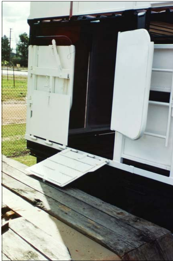
Figure 2 A wide external entry door to a stock crate designed to reduce injury and bruising to cattle
