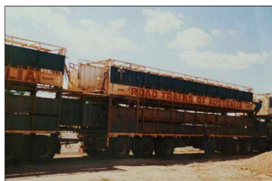
Figure 5 Side view of two adjoining trailers of a road train which are being set up for through loading of cattle
