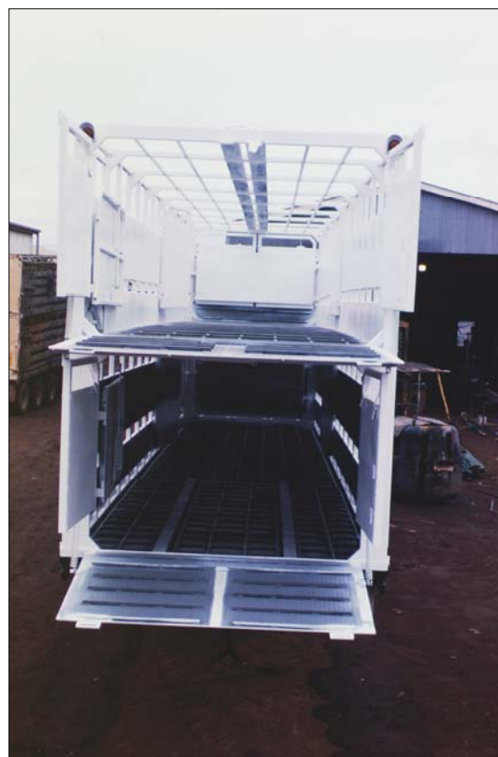
Figure 4 View of a double-deck cattle stock crate with no vertical supports showing a fully opened centre partition that allows through loading of cattle between adjoining trailers on the top and bottom decks
