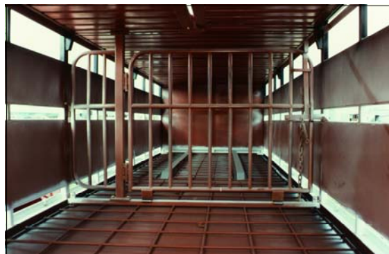
Figure 3 View of the bottom deck of a double-deck stock crate showing no vertical deck supports to avoid bruising to cattle, plenty of gaps in the side cladding to give adequate air flow and a three-quarter width internal division gate
