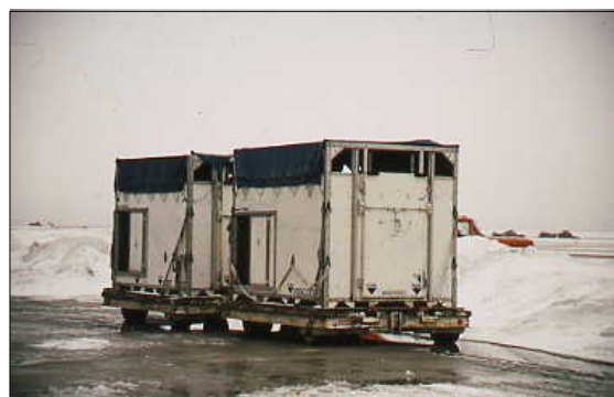
Figure 5 Jet stalls (air stables) on the runway, waiting to be loaded onto an aircraft
