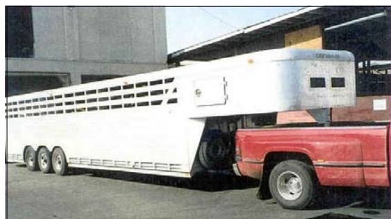
Figure 3 Goose neck single-tier trailer common for the transportation of medium-sized loads of horses to slaughter
