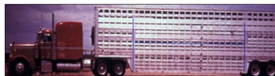
Figure 1 Semi-truck and double-deck trailer ('pot-belly'), with blue lines indicating the principal compartments
