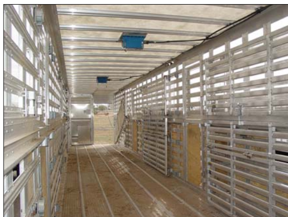
Figure 6 Trailer interior with study cameras on roof in straight-deck trailer
